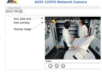
The difference between an overlay and a privacy mask is that a privacy mask cannot be bypassed by accessing the video stream with the help of the AXIS HTTP API, whereas an overlay can.
